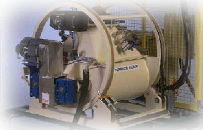
Rotation starts. After the finish of the coating process, the machine turns for discharging. The whole rotation only takes a few seconds..
