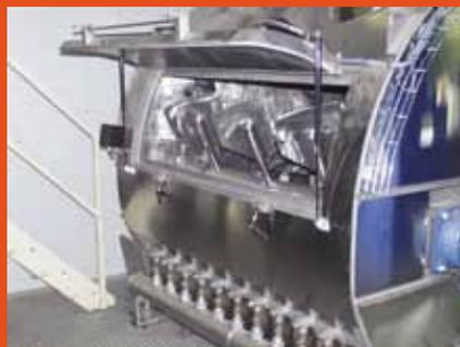
is rotated upside down and the product is discharged through the same opening as for filling. The machine is then rotated back 180° and is ready for a new charge. A feature for the F-RM is the automatic washing and drying of the mixer (Figure 6).
