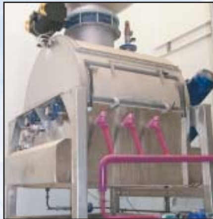
Forberg F-500 conditioner/mixer with steam injection
