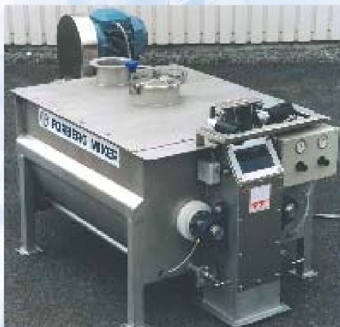
Forberg Continuous Mixer F-120 Conti for testing.
