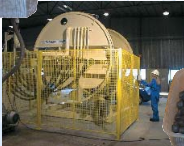
Forberg Vacuum Coater F-3600-RVC during factory acceptance test (FAT)
